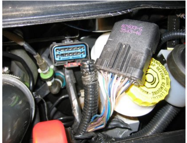
Figure 1: C101 Connector disconnected with harness unwrapped
